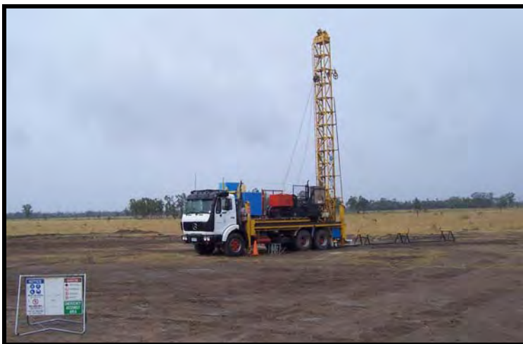
Figures 5 & 6: Drill stem testing with small truck-mounted rig.
