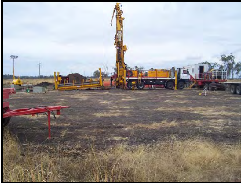
Figure 3: Core or stratigraphic hole drilled with small truck-mounted rig.
